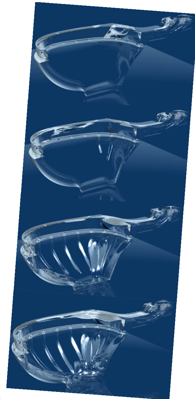
Figure 7. Different time steps during the flushing of a toilet
